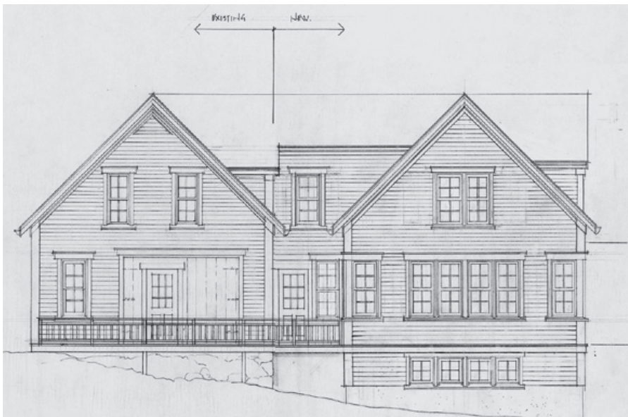
Detail from East Elevation architectural drawing, showing connection between the original 1880 boat shop at left and new addition (courtesy of architect Michael Grunsky)
