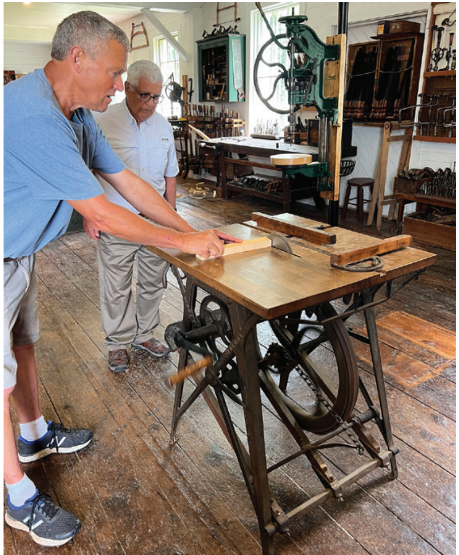
Kevin Wood demonstrating the use of a spring-driven table saw; once the handle is cranked, generating the necessary rpms in the saw blade, cutting can commence, taking care to stand clear of the still rotating handle (photo courtesy of L.E. Omstead)
