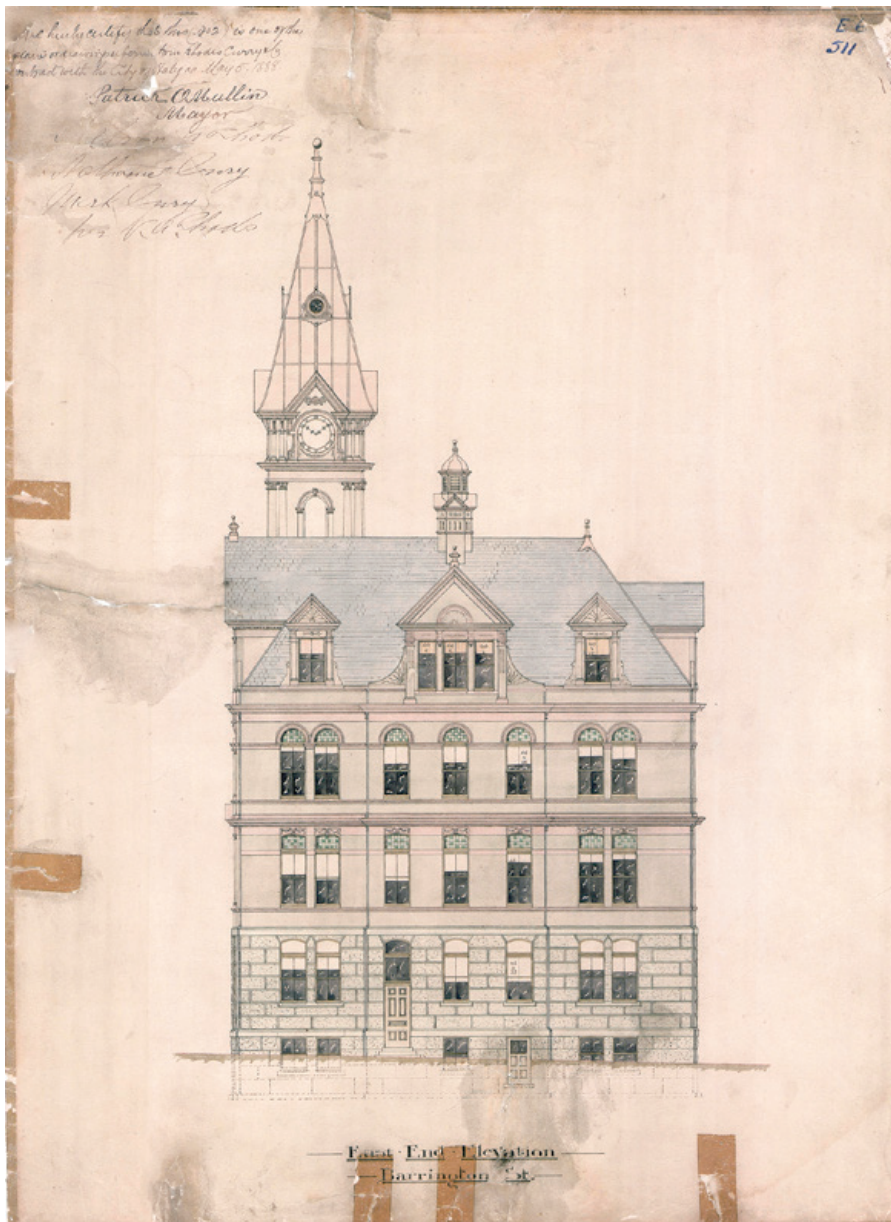
East-end elevation drawing, signed by Mayor Patrick O'Mullin and builders Rhodes and Curry in May 1888, showing basement entrance to Police Department and recessed windows and door in sub-basement (courtesy Halifax Municipal Archives, E-6-511)
