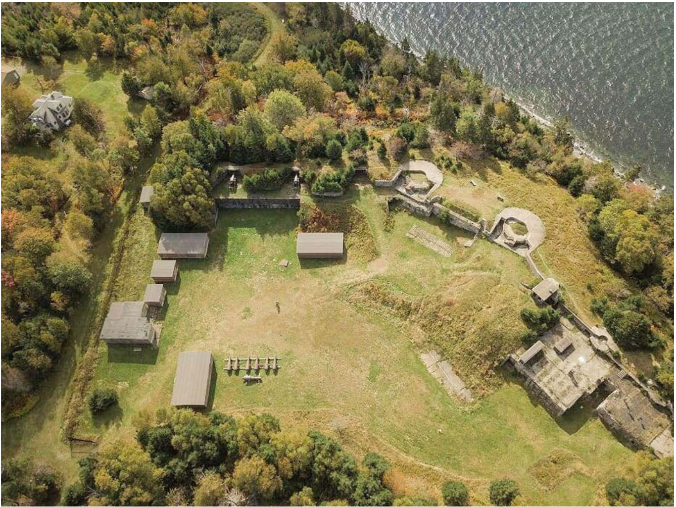
Aerial image of Fort Ives looking southwest, showing retired cannon (lower left of centre), two 10" RML cannon on carriages in emplacements facing southwest (upper left of centre), and emplacements for two 6" BL guns on the west-face obscuring original 9" RML positions (October 2018 image courtesy of Cory Martin)
