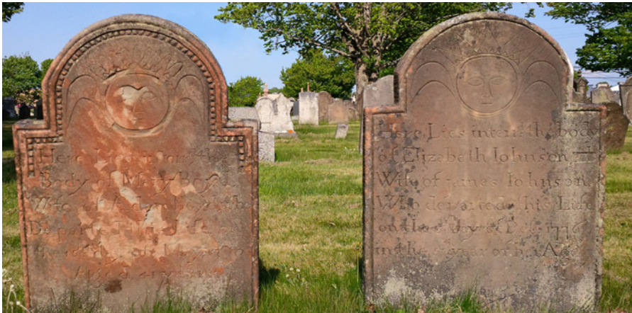
Two of the older monuments in the Robie Street Cemetery, Truro (Mary Boyd, died 1790 aged 41 years and her mother Elizabeth Gourley Johnson died 1776 aged 50 years); note damage caused by misguided cleaning, particularly on the left-hand stone.
