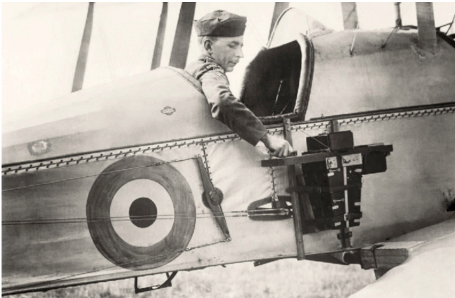
Typical arrangement for air photo camera operations during the First World War (photo Q33850, 1916, from collection of the Imperial War Museum, public domain photo courtesy of UK Government, Wikimedia Commons)
