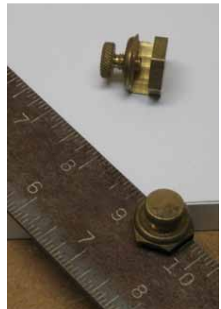
Brass stair gauges can be used while marking angles with a framing square. (Courtesy of Bruce MacNab)
