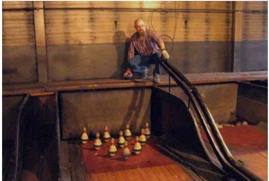
A ball return from atop the pin-monkey runway. Automated equipment was never installed at the Rollways.
